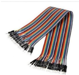
Gambar 2. 10 Kabel Jumper
