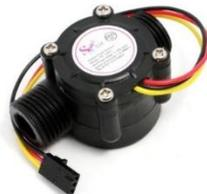
Gambar 2.3 Sensor Flow
