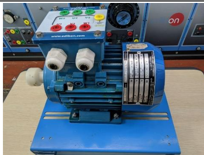
Figure 2. 3-Phase Induction Motor
