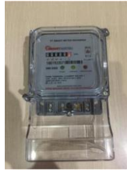
Figure 3. Postpaid semi-digital kWh meter
